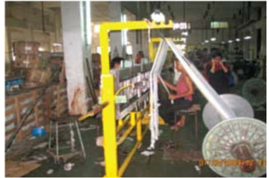
(2) Drawing the warp beam ready for weaving
