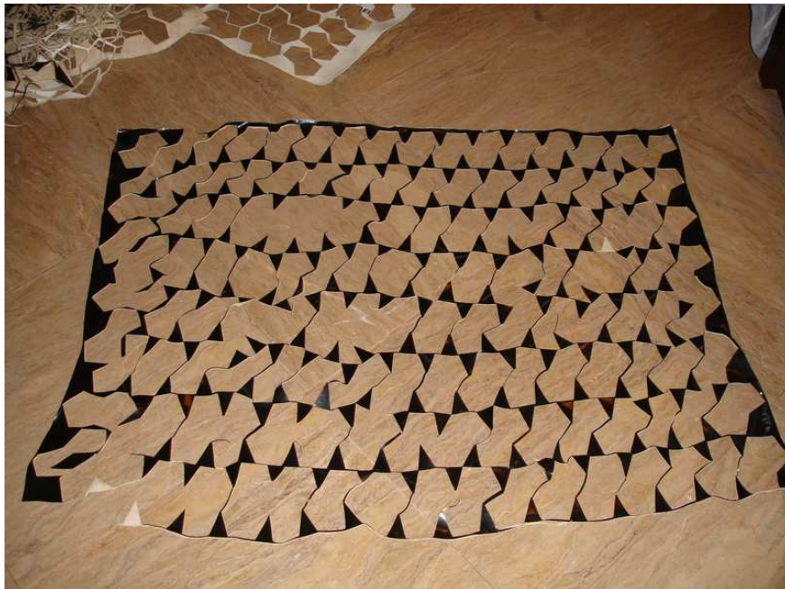
Figure 9: Laminated Sheet Wastage from Cutting Pentagons
