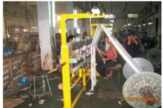
(2) Drawing the warp beam ready for weaving
