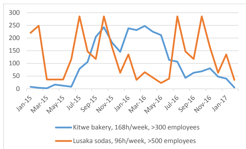
Figure 4 Self-generation hours/month profiles of one large manufacturing firm in Kitwe and one large manufacturing firm in Lusaka, Dec 2014-July 2018. Note: empty bars do not necessarily mean no generation hours that month
