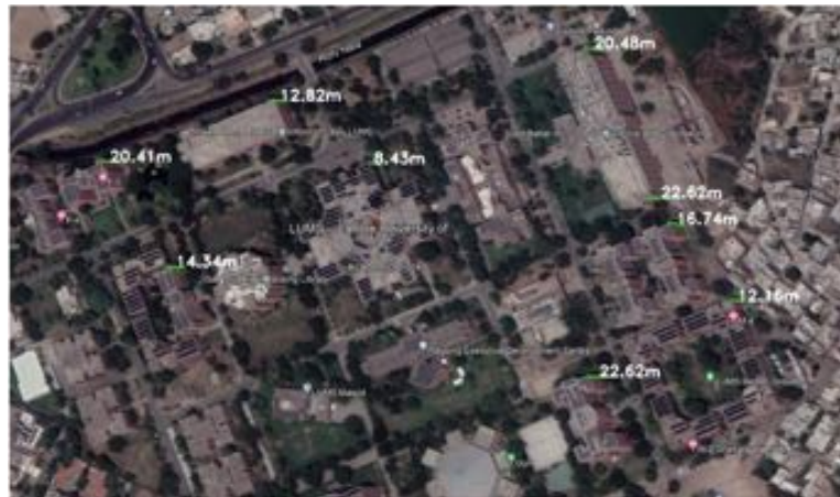
Figure 7: Image showing height estimated by the proposed solution for various building within the LUMS campus.
