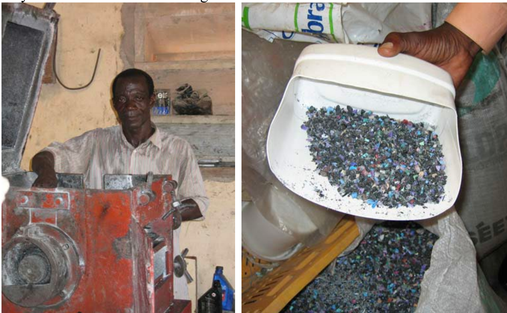
Figure 7. 2: Typical plastic recycling facility with drying benches for cleaned plastic recyclables. Grinder unit and regrind
