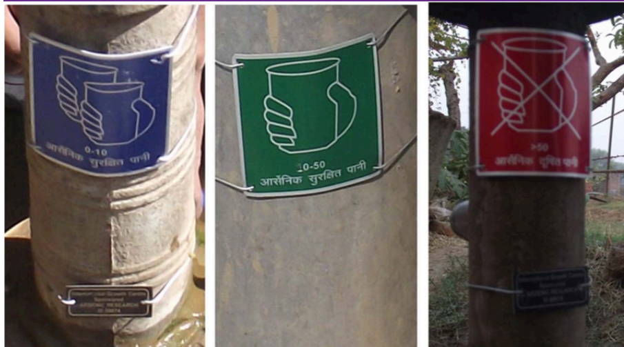
Figure 2: Metal placards with test results attached to pumphead
