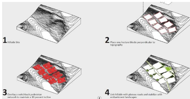
Figure 25 Light Earth Designs, Manual for a Complete Neighbourhood: Flooding Resilience
