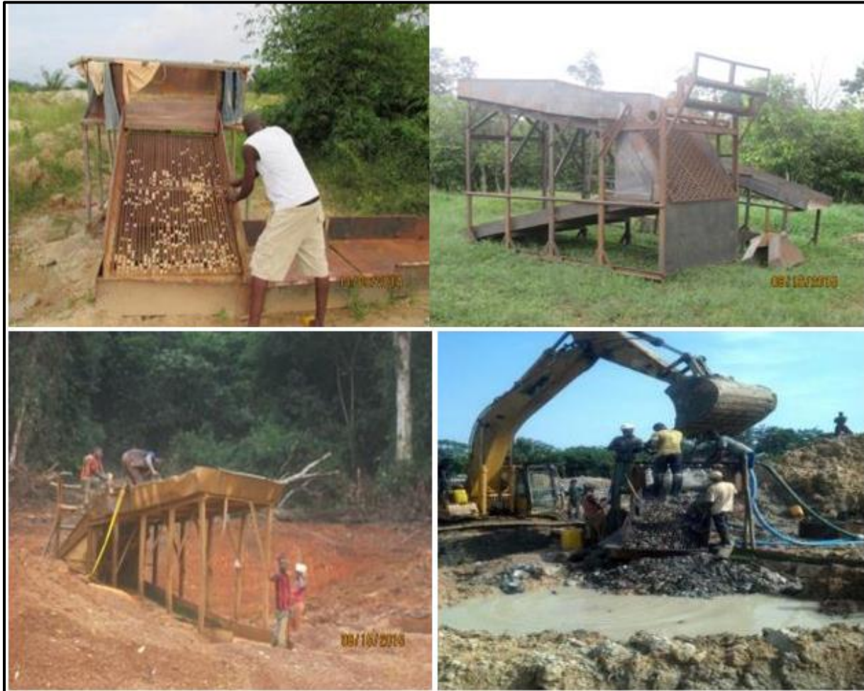
Figure 2: washing board (comes in different sizes/capacities, configurations, set-up etc.) in operation
