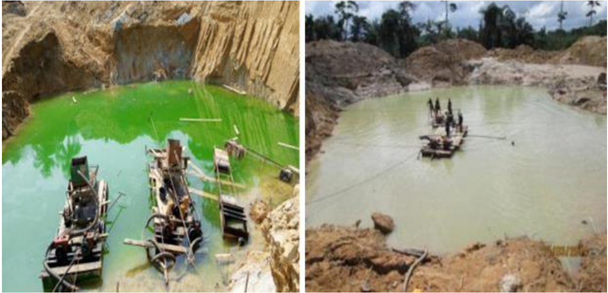
Figure 4: “Anwona” type of operation in abandoned pits created by alluvial washing board operators
