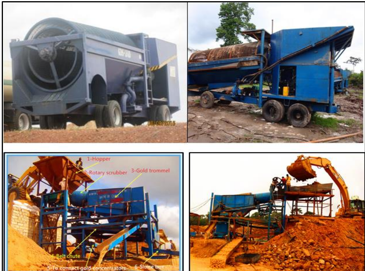
Figure 1: A typical washing plant/trommel
