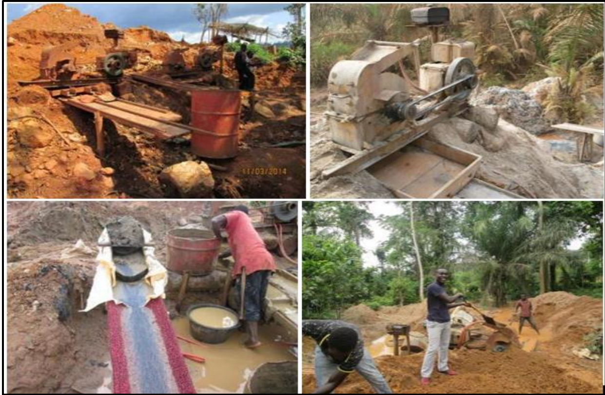
Figure 9: Sluice box fed with “black” (left) at a chamfi site (right) at Mpohor
