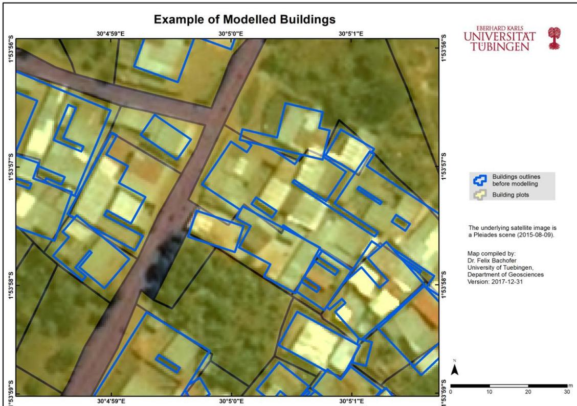
Fig. 4: Automatically detected and generalized buildings. The example shows adjacent buildings treated as single objects.
