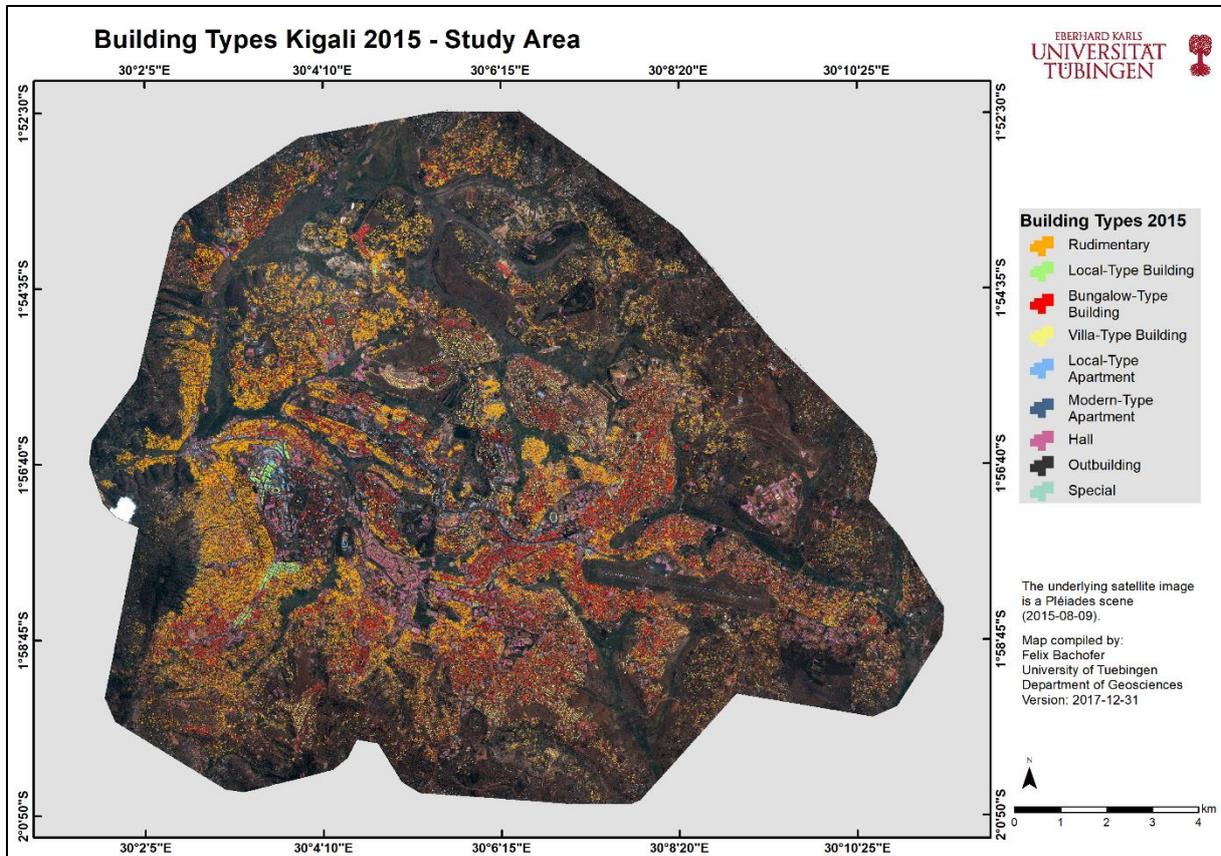
Fig. 17: Result of the building type classification for the study area (2015).
