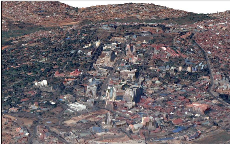
Fig. 6: DSM of the CBD in Kigali. Wide roads and a flat terrain at the CBD in the Nyarugenge sector led to good results in this part of the city.
