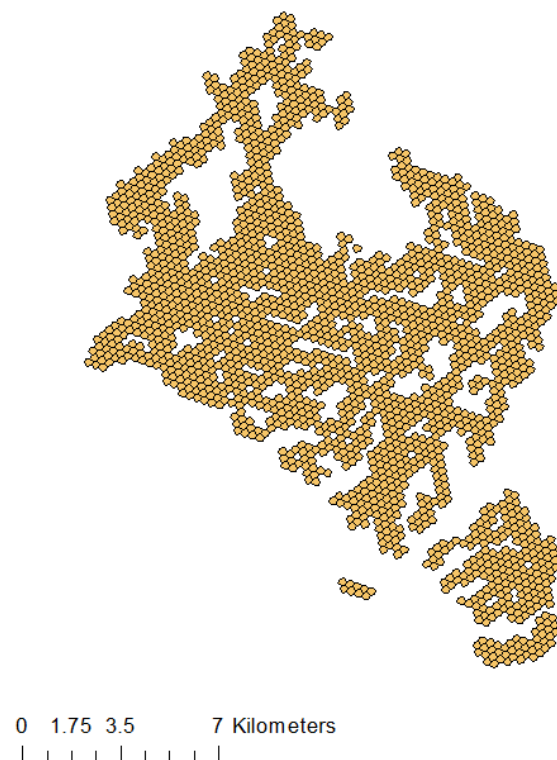
Hexagonal Zones (150 Meter Sides, 300 Meters in Diameter)
