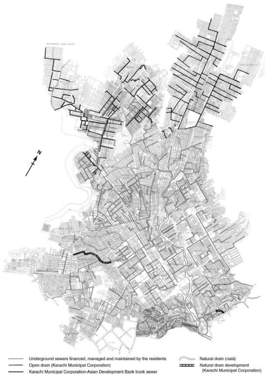
Figure 9: The sewers in Orangi, Karachi, financed, managed, and maintained by the residents 38
